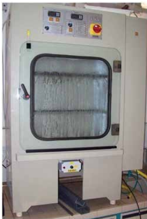
Figure 45.1. Erichsen Mod. 519/AUTO Cyclic corrosion cabinet (by the authors, 2011).
